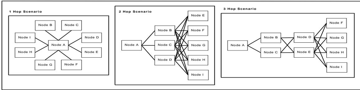
Figure 2. Topological view and connectivity of one hop, two hop and three hop scenarios.
