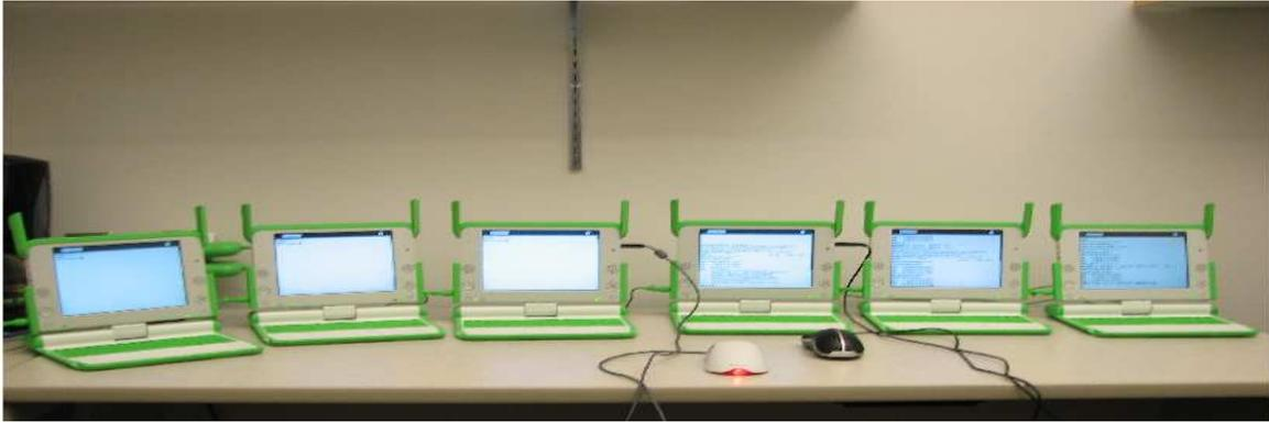
**Figure 1. Six of the OLPC XOs that are currently used as MANET nodes at the University of Victoria.**
